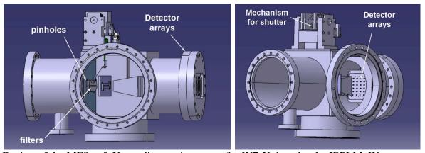
Design of the MFS soft X-ray diagnostic system for W7-X done by the IPPLM, Warsaw.
