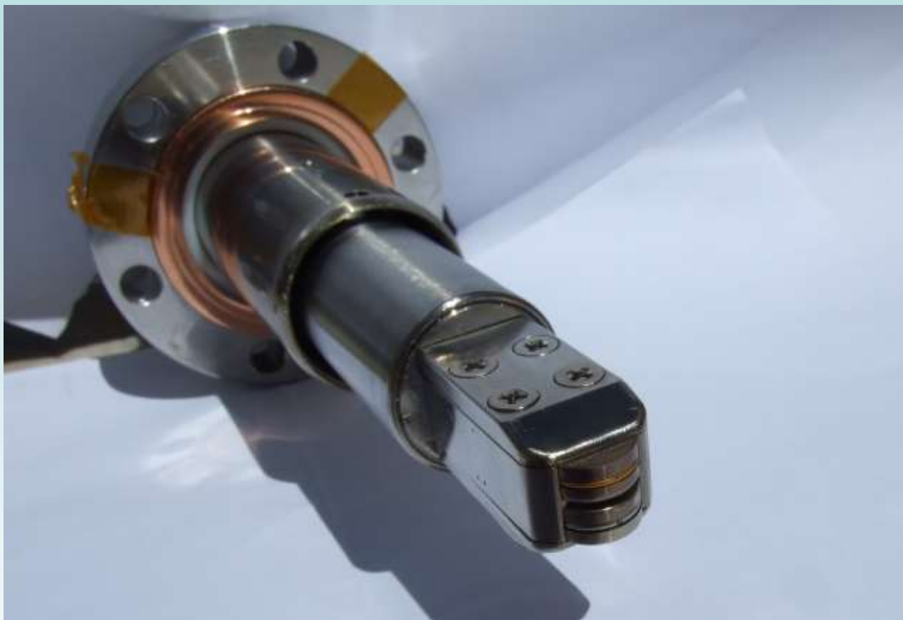
The view of the new, two-channel measuring head of the Cherenkov probe dedicated for measurements of electron beams within the ISTTOK experiment
